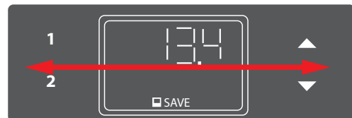
Fig. 51. The LegaDrive Touch Inlay handset lock is activated and deactivated by swiping to the left or right
